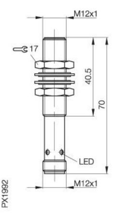
Inductive Sensors BES 516-325-S 4-C M12x1 x 70 normally-open Sn=2mm shielded
